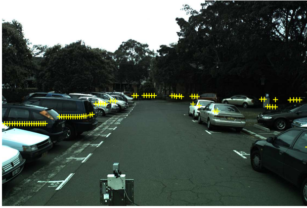
Fig. 6. Reference scene (left) and scene 91 (right) with projected laser point (gray/yellow crosses). CRF matching identifies this scene as the best match indicating the most probable position where the loop closure occurred. Note that the laser scans are substantially different.
