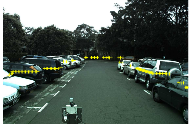
Fig. 6. Reference scene (left) and scene 91 (right) with projected laser point (gray/yellow crosses). CRF matching identifies this scene as the best match indicating the most probable position where the loop closure occurred. Note that the laser scans are substantially different.
