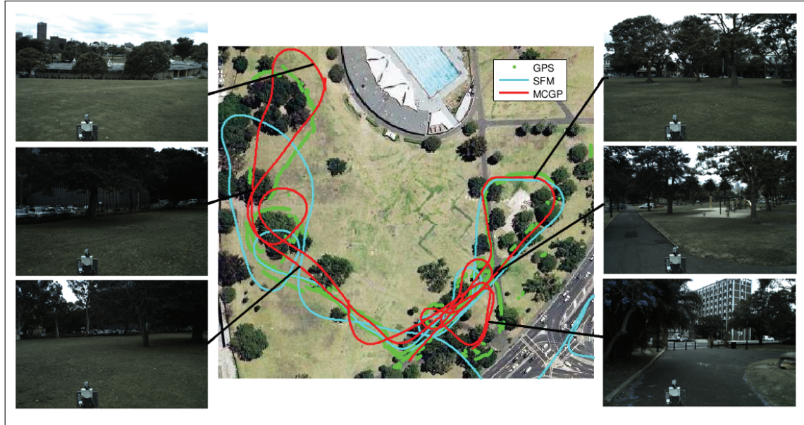
Fig. 11. Localization results in off-road ground experiments.
