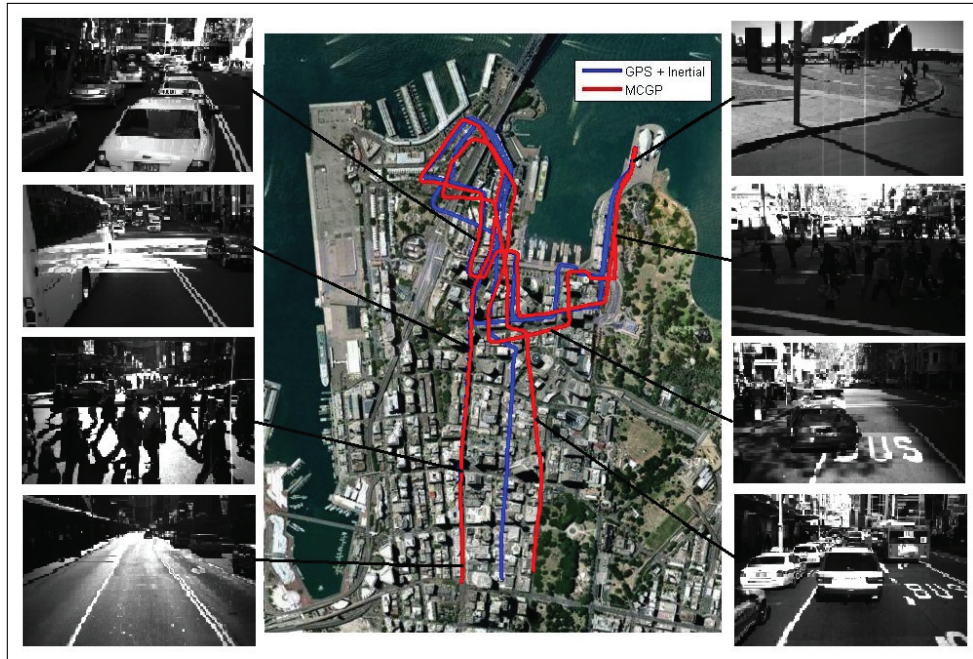
Fig. 15. Localization results obtained using the proposed method and a different robotic platform (training and testing conducted in the same conditions), along with sample images obtained during navigation.
