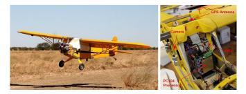
Fig. 1. The autonomous UAV, based on a J3 Cub 1/3 scale model. Sensor payload includes IMU, GPS receiver, downward pointing monocular camera and a PC104 stack.
