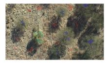
Fig. 3. A visualisation of some of the manual labels provided to the classifier, with colour overlays indicating segments that have been labeled for each class. A total of 160 such sparse samples (40 of each class) were drawn over 32 manually selected frames to build a training set.
