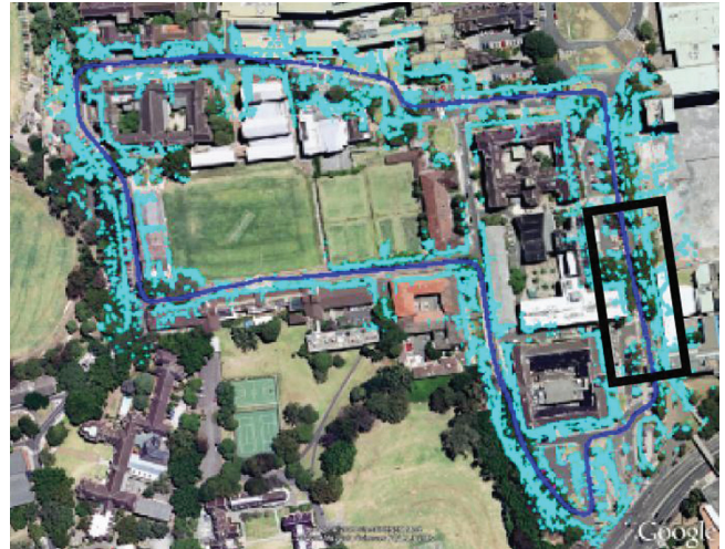
Fig. 15. Satellite view of scanned region with laser returns indicated.
