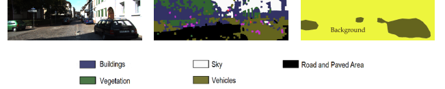
Fig. 4: Left image shows the raw image, middle overlays output of the pLDA classifier. Right image present the recognised foreground objects using the FCN classifier
