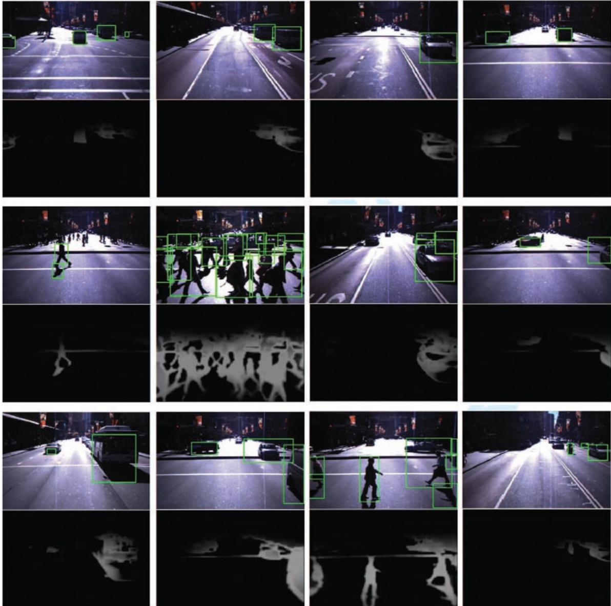
**Fig. 14.** Different object instances obtained during the iterative clustering process.
