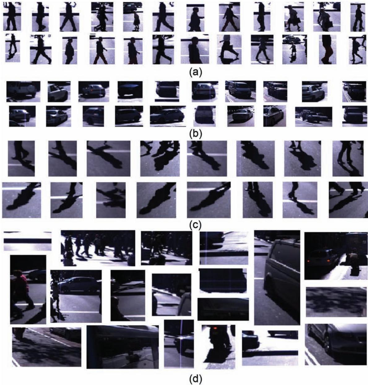
**Fig. 15.** Clustering results for different dynamic objects. (a) Pedestrians. (b) Vehicles. (c) Pedestrian shadows. (d) Examples of objects that do not belong to any of the three main categories.
