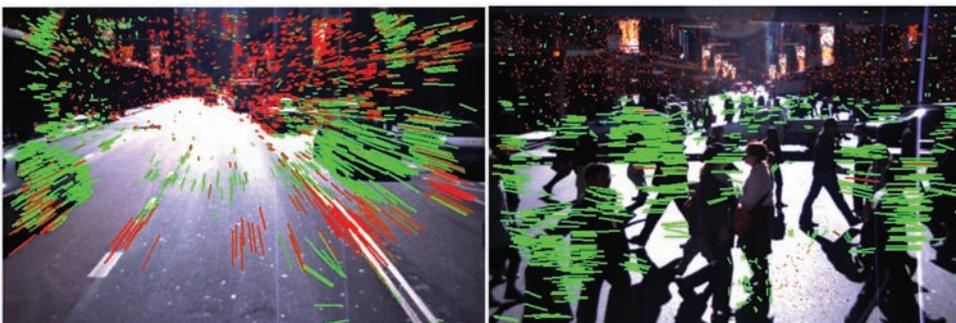
**Fig. 4.** Initial RANSAC classification, based on the image information presented in Figure 2. Each line segment has a color ranging from red (static object) to green (dynamic object), and matching pairs considered outliers were discarded.
