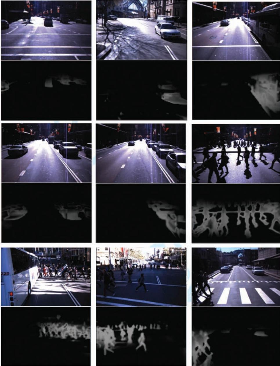
**Fig. 9.** Final segmentation results. Each pixel is defined by a number ranging from 0 (black, static object) to 1 (white, dynamic object). These results were obtained in the same run as the non-parametric model constantly adapts to new environment characteristics, without any prior information and without any human intervention.
