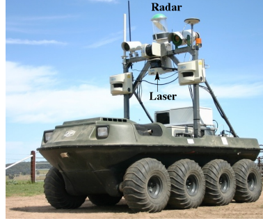
Fig. 2 Argo UGV equipped with the laser and radar sensors used in this study.
