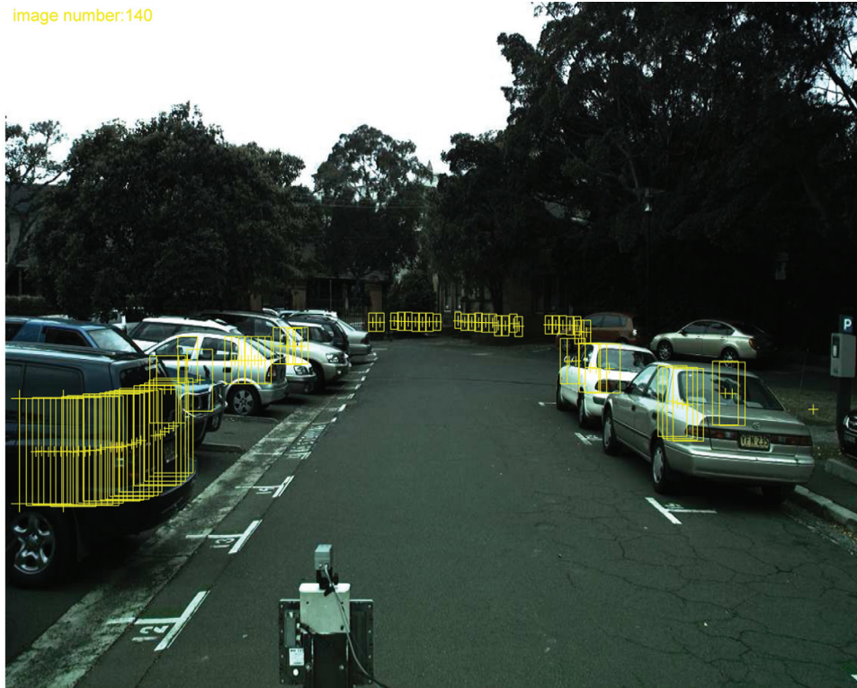
Fig. 9. Examples of ROIs generated by the system. The ROIs are indicated by the yellow rectangles, the laser returns are indicated by the yellow crosses at the center of the rectangles. It can be seen that the size of the ROI is decreased for longer ranges. As discussed in Section 3.2, the fact that these ROIs overlap and generate feature vectors with an overlapping content is not a problem from the point of view of a CRF. Since a CRF is globally conditioned on the set of observations, it can readily integrate the content of overlapping feature vectors.
