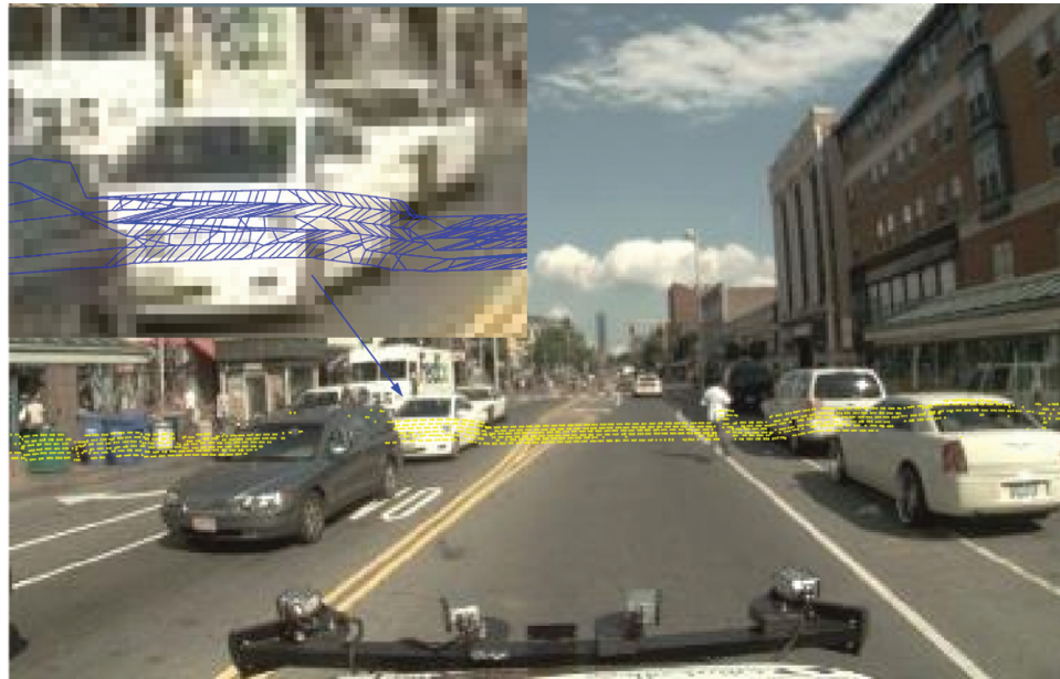
Fig. 11. An example image from the Boston dataset displayed with the associated projected laser returns (in yellow). A part of the CRF network built from these laser returns is displayed in blue in the inset in the top left corner. The labeled scan is that forming the upper side of the network. The image in this inset corresponds to a magnification of the area indicated by the arrow. This figure also illustrates the low resolution of the image, notably with respect to the images in the Sydney dataset (see Figure 10).
