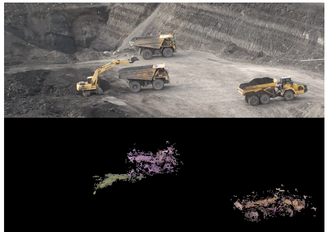
Fig. 9: Moving segments of mining dataset. This shows all moving parts of the scene has been accurately detected. The truck undergoing loading is stationary.
