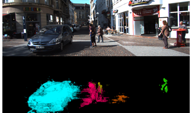
Fig. 1: Example detection of multiple dynamic objects discovered using our proposed method that corresponds to the input image sequence shown above. The different colours (hue) in the output image represents the multiple object instances detected, while the intensity denotes the likelihood of the assigned class at each pixel. These objects were detected using only the motion of the scene and not any off-line models describing the visual appearance of the objects.
